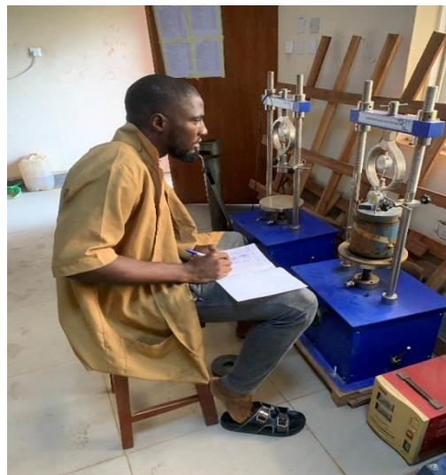
Plate 3.7 Observing and recording the penetration readings
