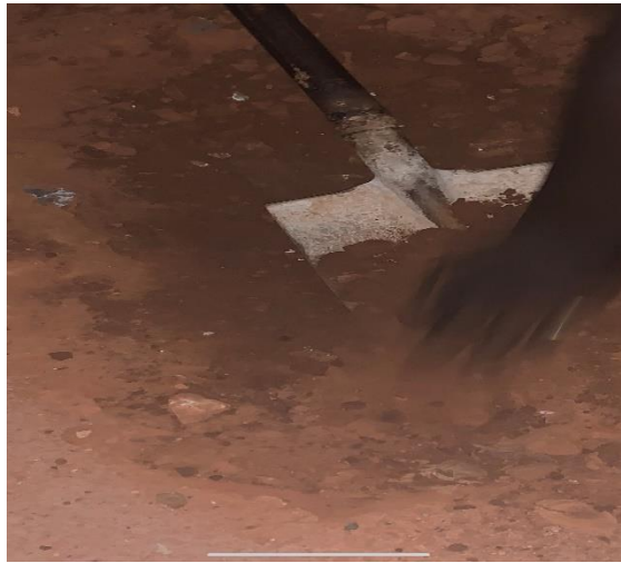
Plate 3.0 The Subgrade soil made up of different particle sizes
