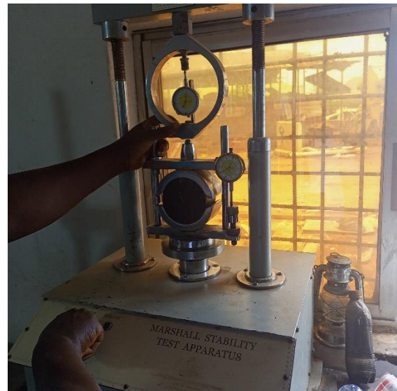
Plate 3.5: (A) Specimen placed in the water bath, (B) Specimen placed in the Marshall Stability testing machine.
