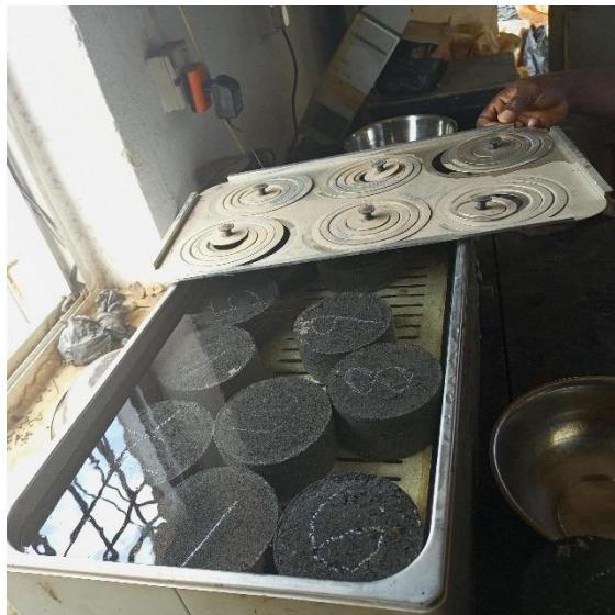
Plate 3.5: (A) Specimen placed in the water bath, (B) Specimen placed in the Marshall Stability testing machine.
