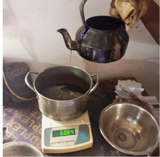
Plate 3.4: (A) Aggregate weighed, (B) Addition of bitumen to the aggregates
