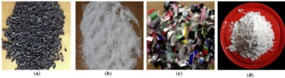
Figure 2.6. Various forms of waste plastics used as modifiers: (a) pellet (Fang et al 2014); (b) shredding (Modarres, and Hamed, 2014); (c) flake; (d) powder (Balasubramanian, B 2021).
