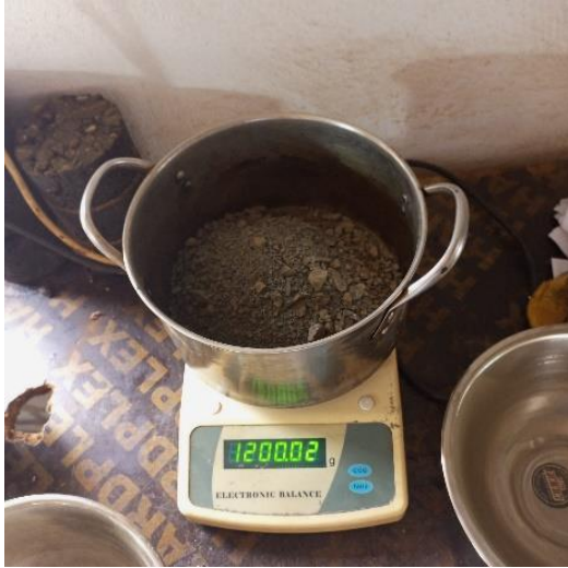
Plate 3.4: (A) Aggregate weighed, (B) Addition of bitumen to the aggregates
