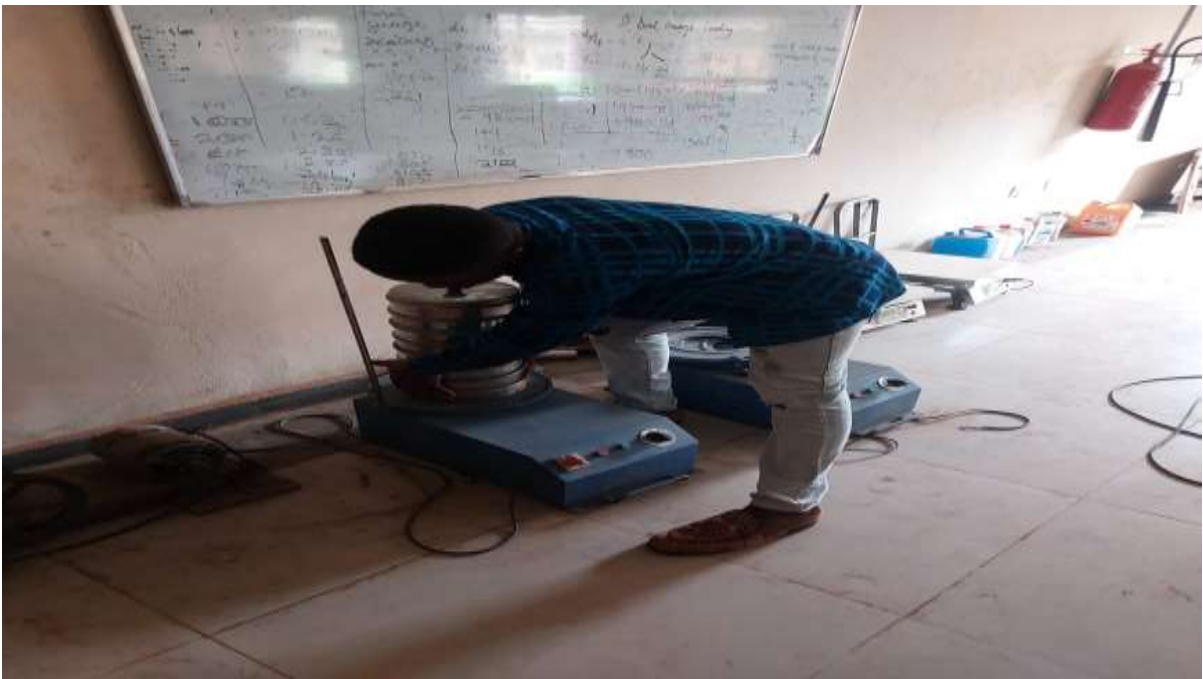
Plate 3.3: Arrangement of Stack of Sieves on a Mechanical Sieve Shaker
