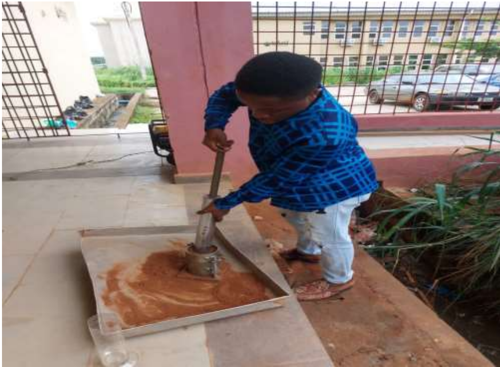
Plate 3.6: Manual Compaction of Soil Sample
