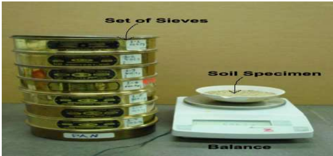
Plate 3.2: Apparatus for Particle Size Distribution Test Source: (Braja,2006).
