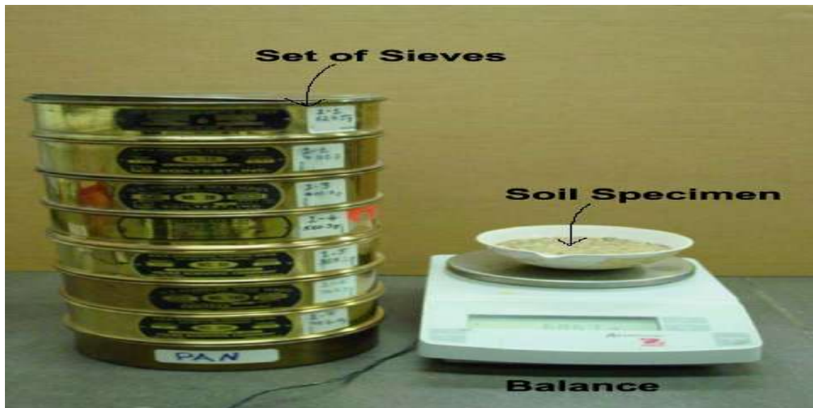
Plate 3.3 Apparatus for Particle Size Distribution Test (Source: Braja, 2006).
