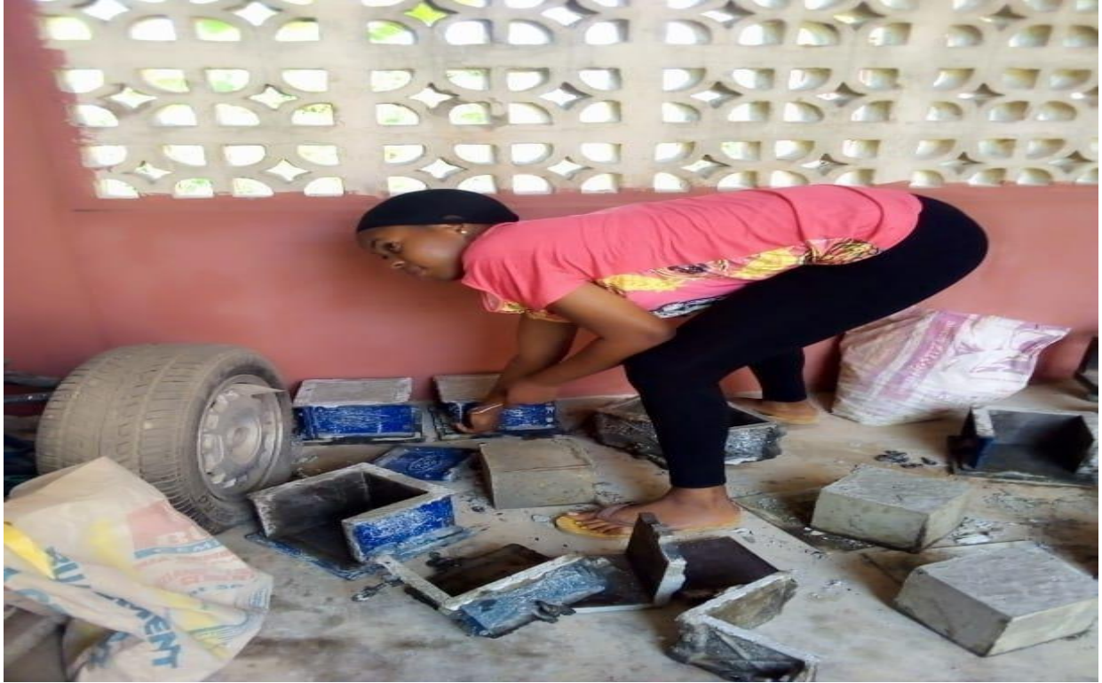
Plate 5: Getting Cubes Ready for Curing.
