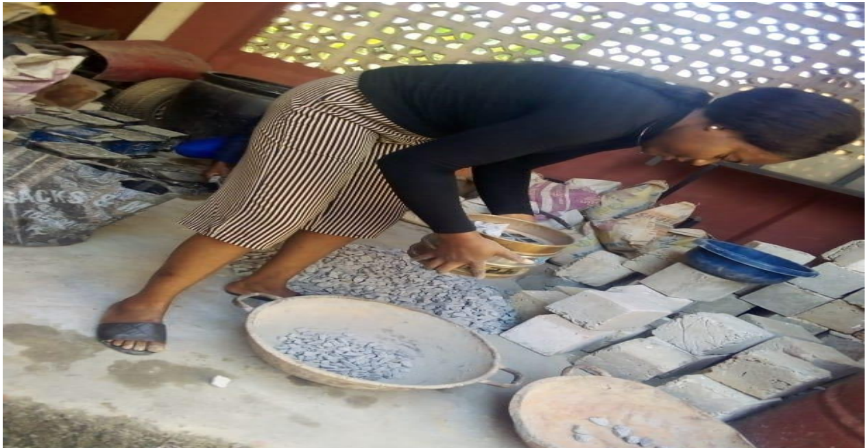
Plate 2: Sieve Analysis on 20mm Coarse Aggregate.
