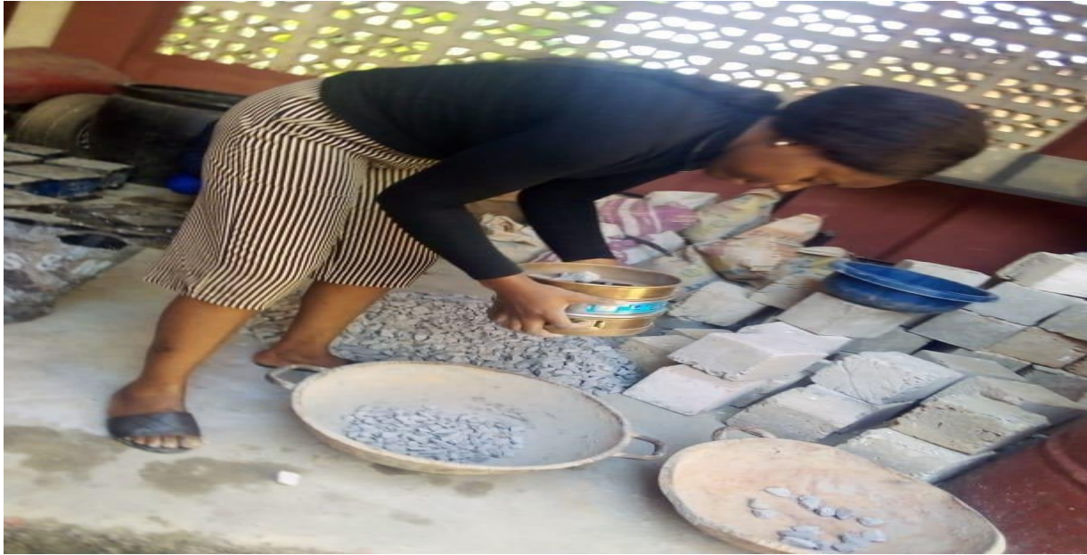
Plate 1: Sieve Analysis on Coarse Aggregate.
