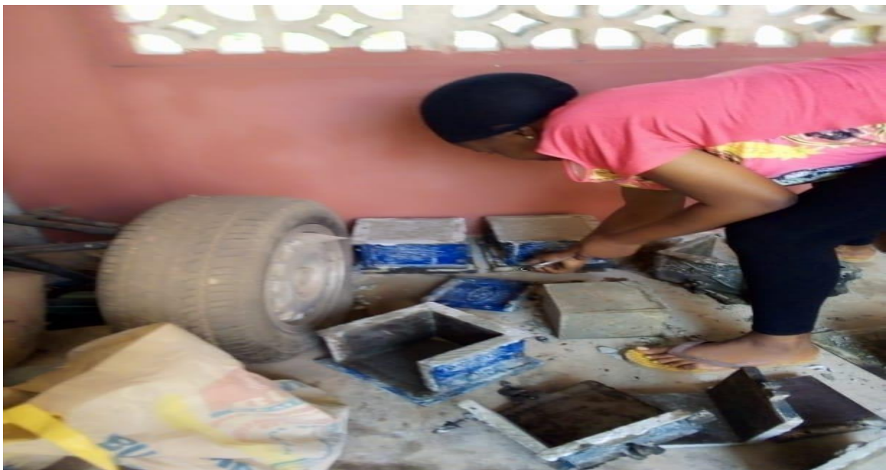
Plate 4: Removal of Cubes from Metallic Molds
