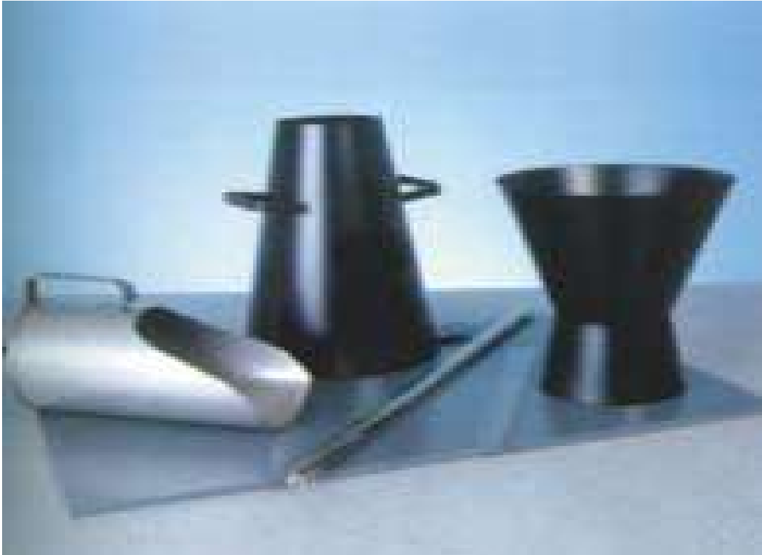
Figure 3.8: Apparatus used for Slump Test
