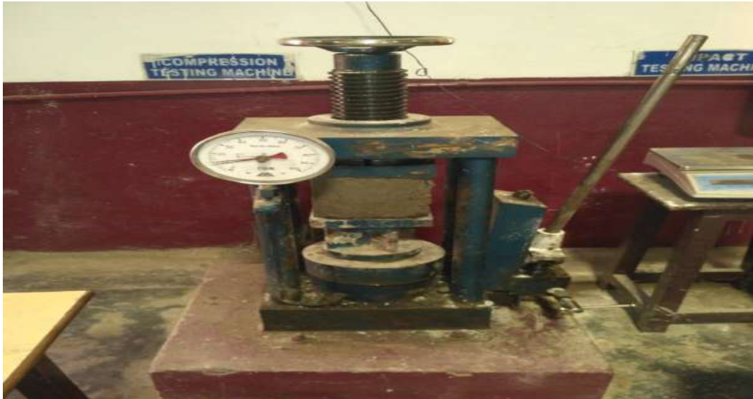
Plate 3.9: Universal Testing Machine for Compressive Strength Test.
