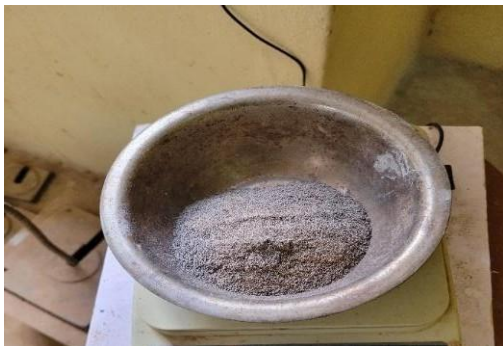
Plate 1: Processed groundnut shell ash used in the study
